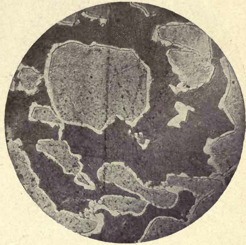
Fig. 12. Alloy D. Cu 78.0 Quenched from 565° C. Sn 22.0 Three phases.
